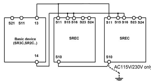
**Fig. 2: Connection of several SREC units to basic device**
