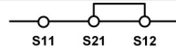
Fig. 10: Automatic start (e.g. for application with a safety door). Max perm. delay during closing of the safety switches on S12 and S13: S12 before S13: 300 ms; S13 before S12: any
