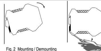
Fig. 2 Mounting / Demounting
