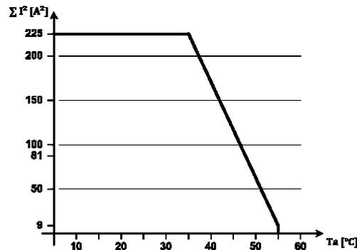
Max. cumulative current depending on the ambient temperature for AC 115 V / 230 V variants with 10 mm space between the devices
