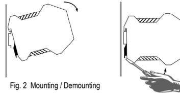
Fig. 2 Mounting / Demounting
