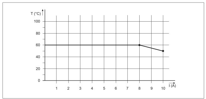
PSSu H PLC2 FS SN SD(-T): Derating diagram for periphery supply: Permitted ambient temperature T dependent on load current I
