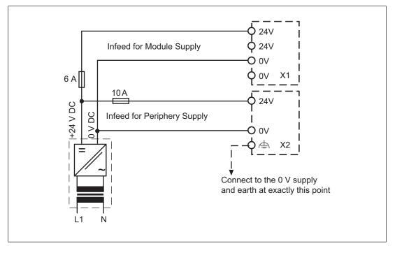
Common power supply for module supply and periphery supply:
