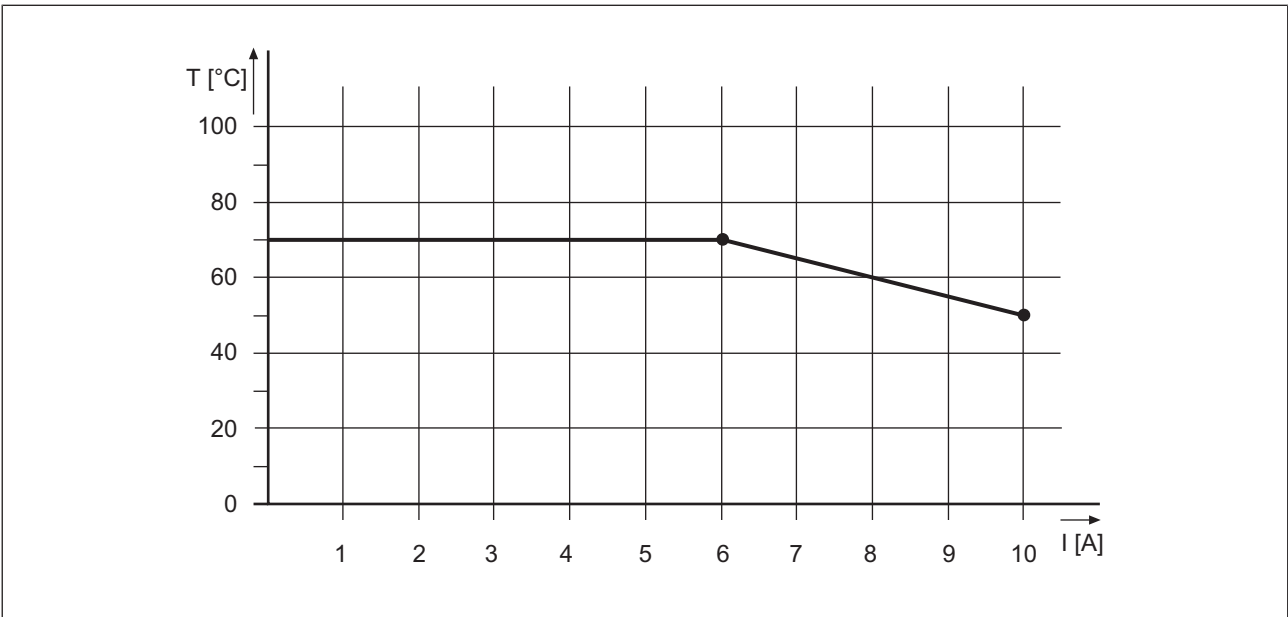
PSSu E F PS-T: Derating diagram for infeed for module supply: Permitted ambient temperature T dependent on load current I
