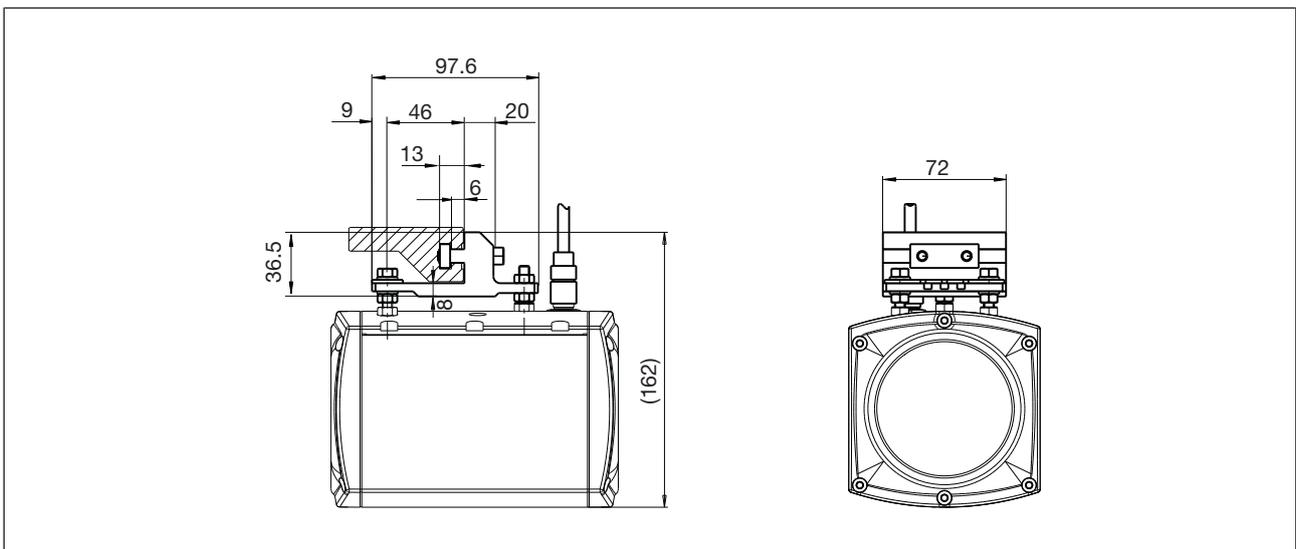
Fig.: Dimensions of the fastening kit for the transmitter, dimensions in mm
