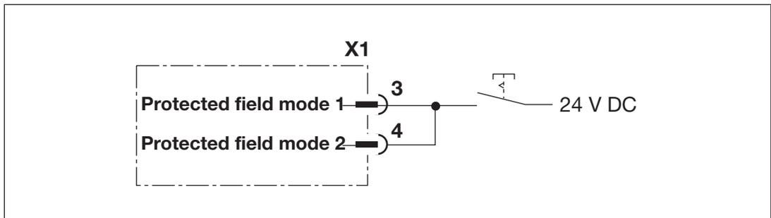
Fig.: Protected field mode 1/2 directly at the 24 V DC supply
