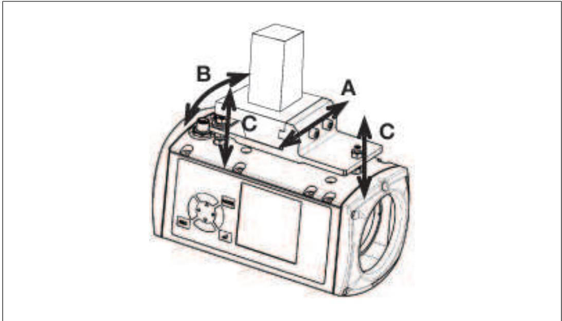
Fig.: Adjustment directions of transmitter and receiver
