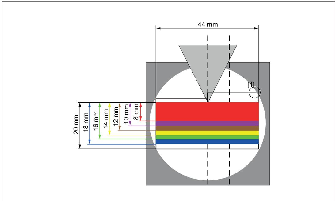
Fig.: Required protected field based on the overrun
