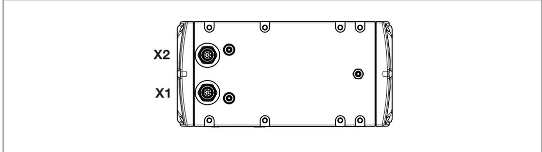
Fig.: M12 connector on the receiver
