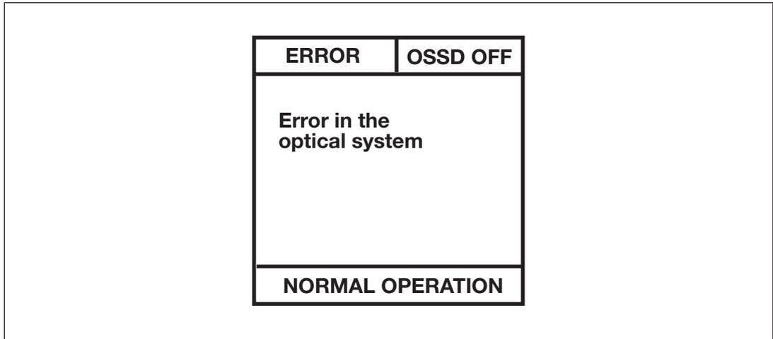
Fig.: Error messages on the display
