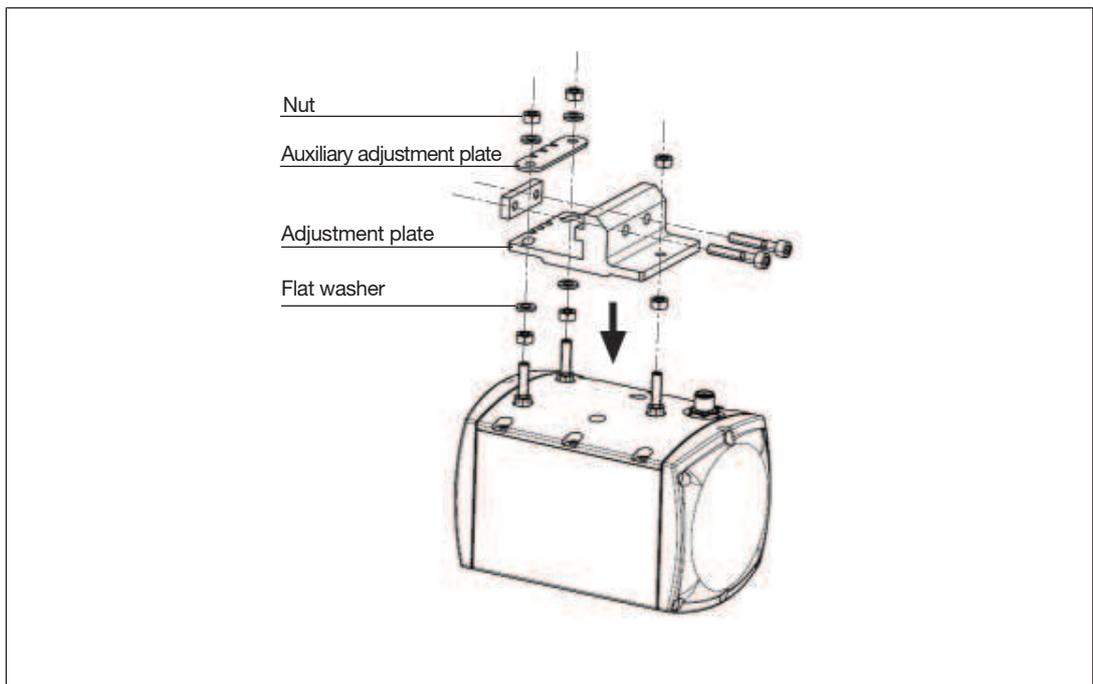
Fig.: Installing the transmitter and receiver
