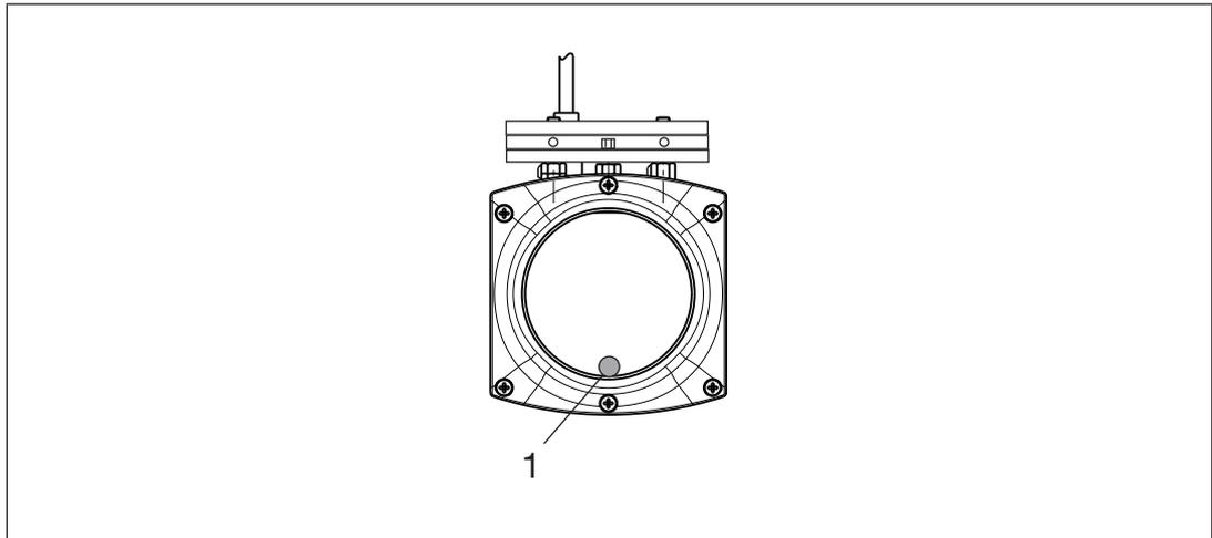
Fig.: LED on receiver
