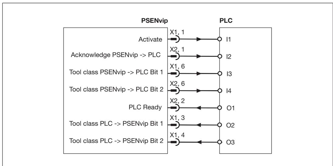
Fig.: Digital inputs and outputs for communication
