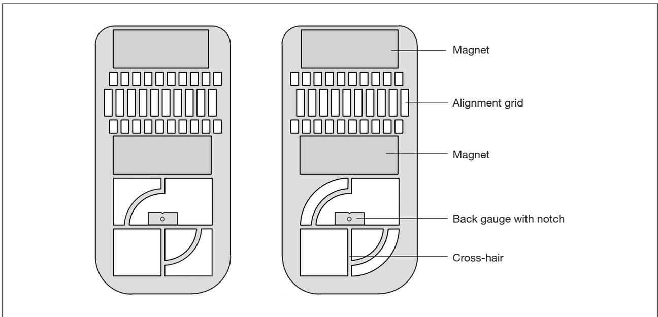
Fig.: Adjustment templates (viewed from the magnet side)
