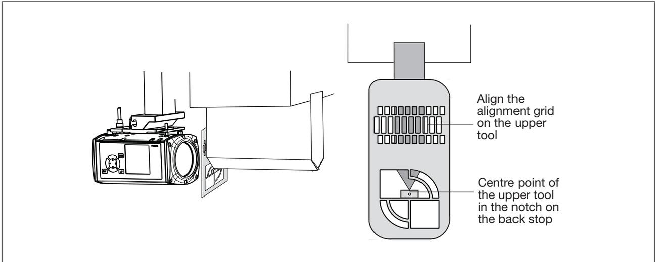
Fig.: Attach the adjustment template to the receiver
