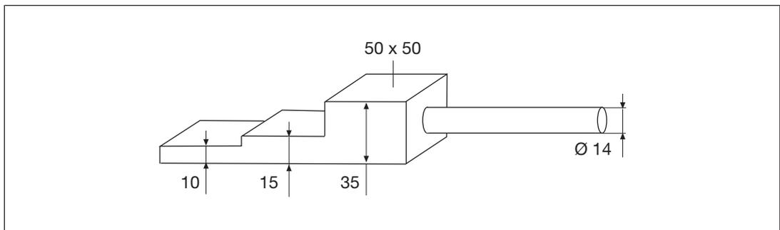
Fig.: Test piece in accordance with EN 12622
