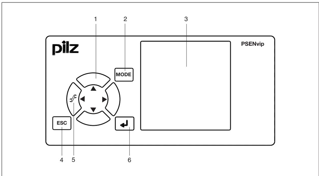
Fig.: Display on the receiver
