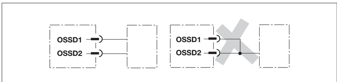
Fig.: Correct and incorrect connection of OSSD1 and OSSD2
