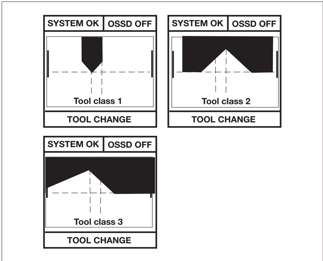
Fig.: Tool detection on the PSEnvip display
