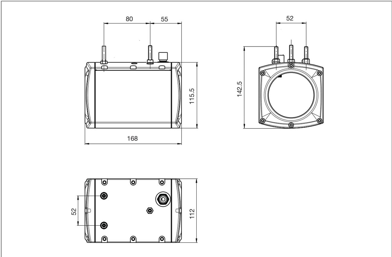
Fig.: Transmitter dimensions, dimensions in mm
