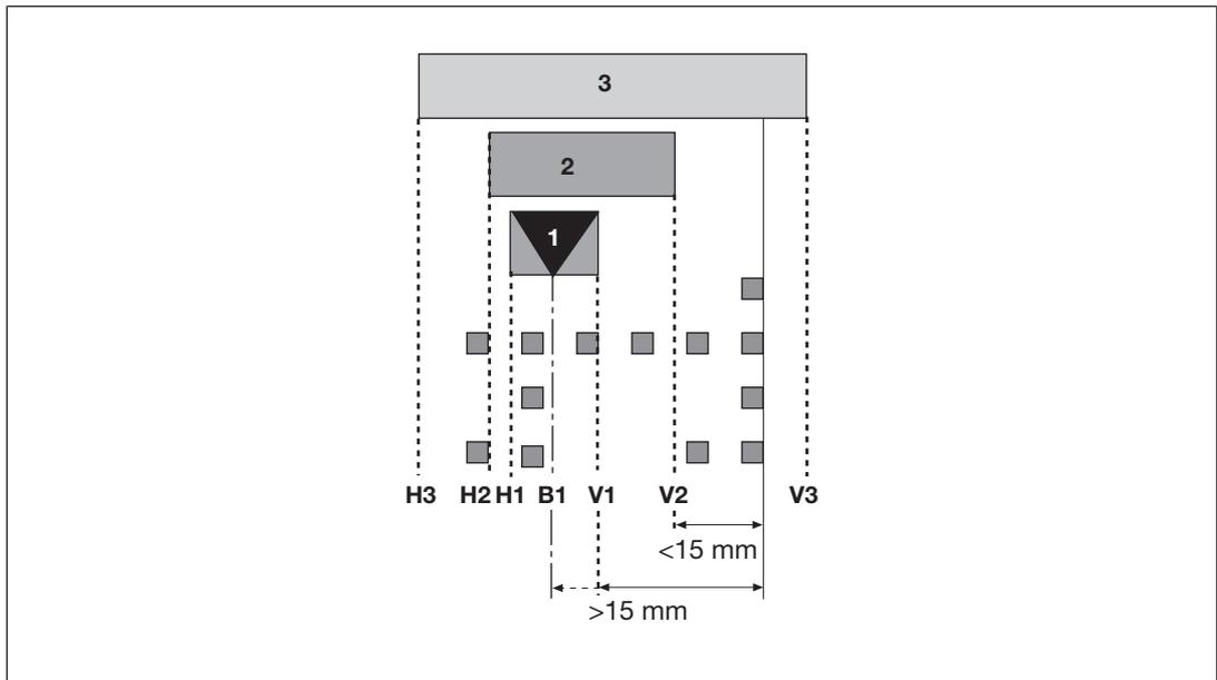
Fig.: Classification of tools into tool classes
