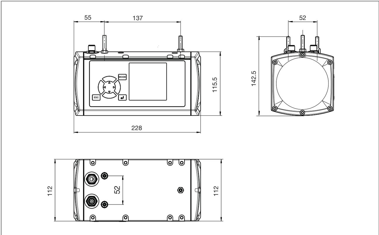
Fig.: Receiver dimensions, dimensions in mm
