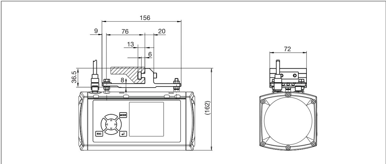
Fig.: Dimensions of the fastening kit for the receiver, dimensions in mm
