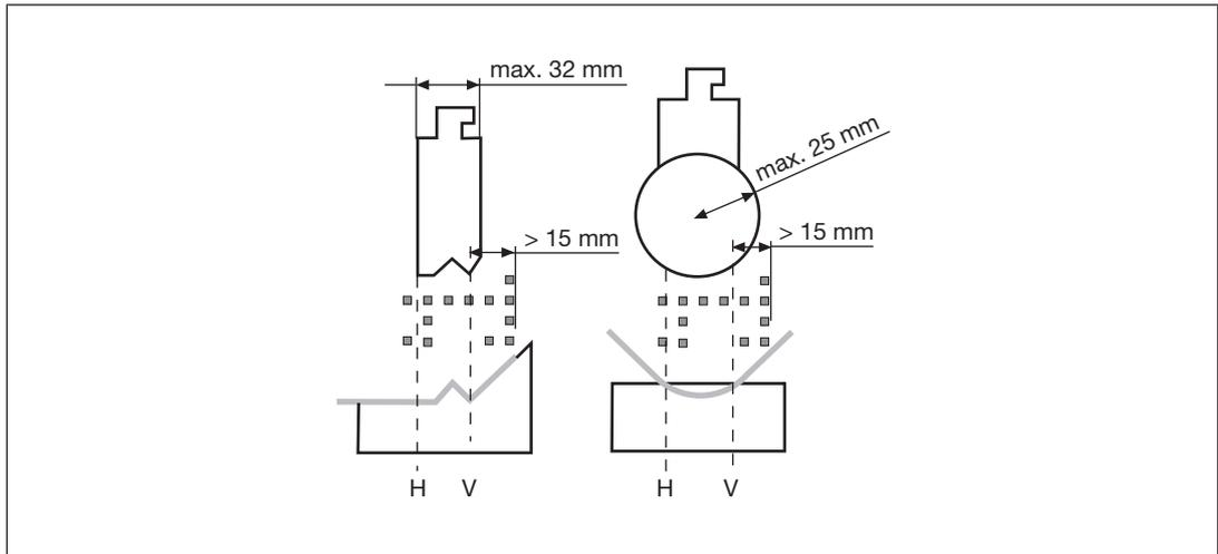
Fig.: Example for tool class 1
