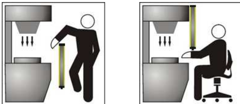
Fig. 5 – Device positioned incorrectly
